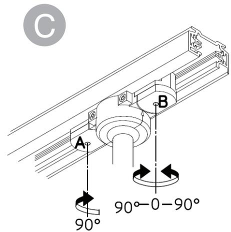
Turn knob **A** clockwise 90° to connect the adaptor to the neutral circuit.
